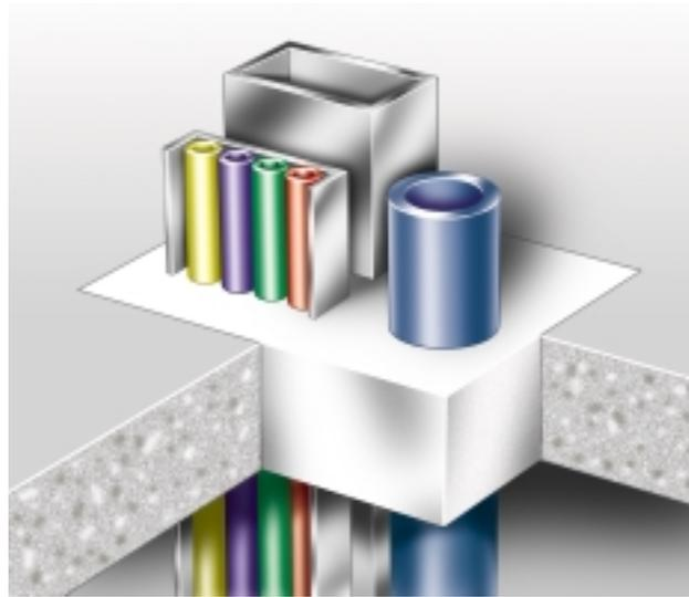
**Fire Rated Load Bearing Mortar system for up to 6 hours protection to compartment floors and walls around service penetrations.**
